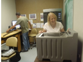
Rachel Watson at the SCA (Support Cleaning Apparatus), a heated chemical bath to remove the support material used in the Dimension Elite 3D Printer, seen in the background.
